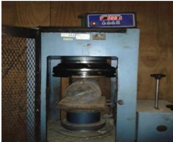
Figure 1: Test setup of split tensile strength
