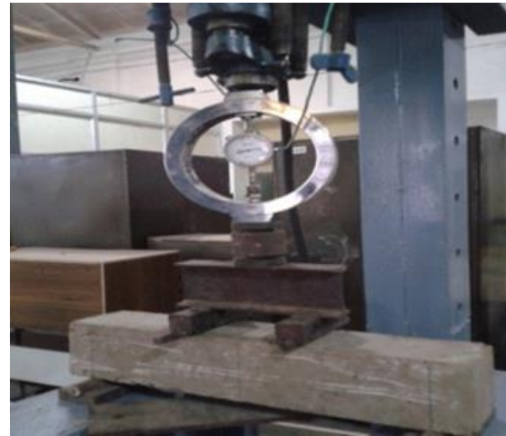
Figure 2: Test setup of flexural strength
