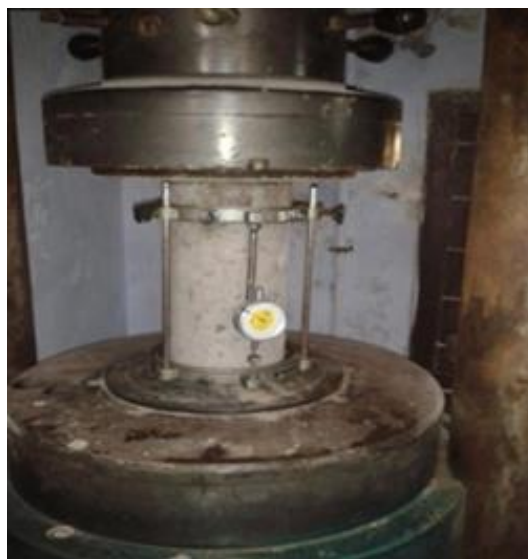
Figure 3: Test setup of modulus of elasticity
